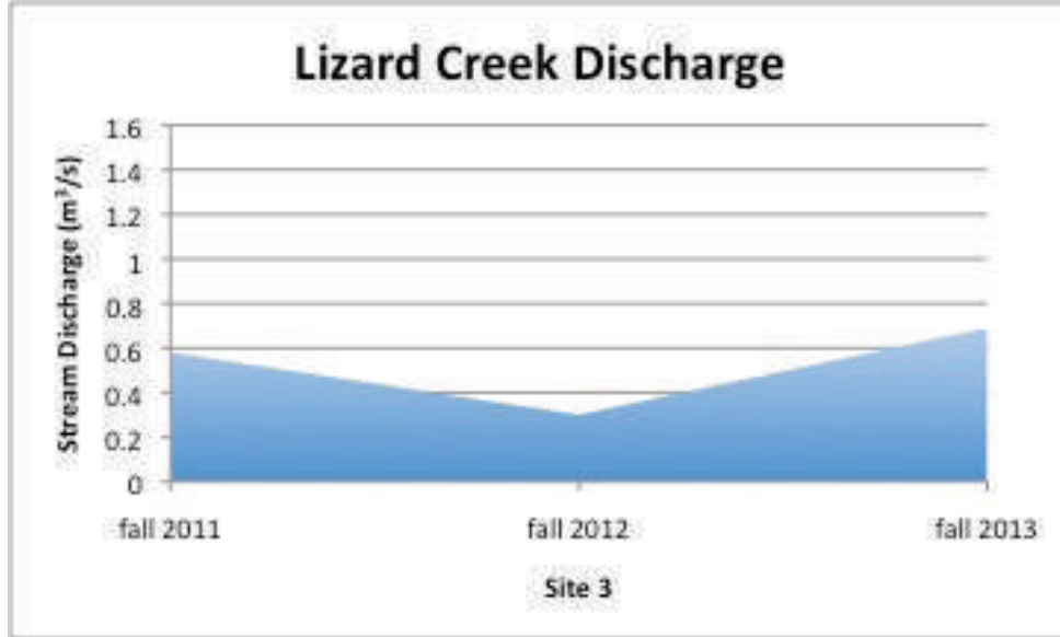
FIGURE 17. Lizard Creek site 3 low flow stream discharge (m 3 /s), calculated by multiplying the cross-sectional stream area (m 2 ) by the velocity (m/s), results range from 0.3-0.7 m 3 /s
