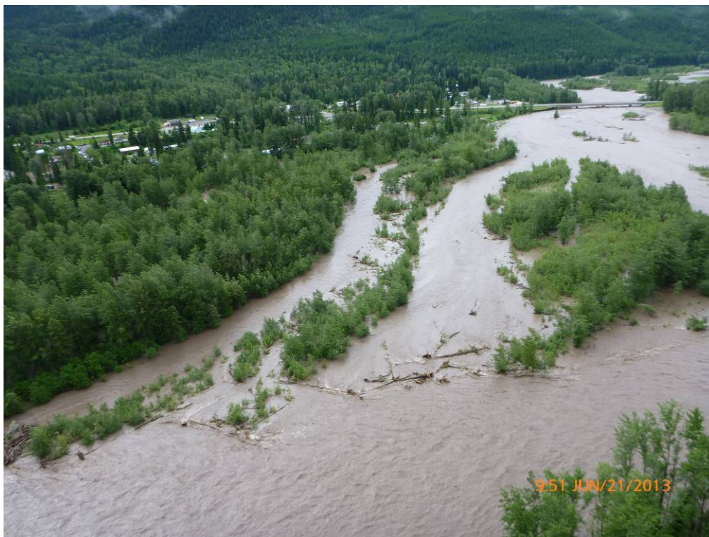
Figure 8. Downstream view of wide flooded area backwatered by Highway 3 (Source: RDEK).
